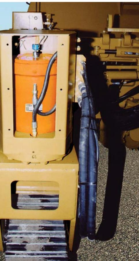
**Even if Helac's L-30 series rotary actuator didn't provide a simpler, more compact design than conventional steering cylinder assemblies, its steering angle is more than twice that of cylinders — still making it an attractive alternative.**
